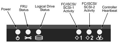
Figure 1. VTrak M500f/i/p front panel LED display
